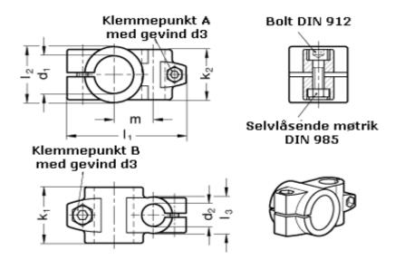
Adjustable clamp lever for d3 = GN 911-M 8-32 have to be ordred separately Adjustable clamp lever for d4 = GN 911-M 6-25 have to be ordred separately d1 = 25 d2 = 18
